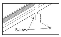
Remove the bolt from the upper end of each handrail.
